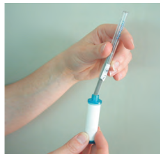
1. Transfer adsorbent cartridge from the storage container into the diffusive body.
