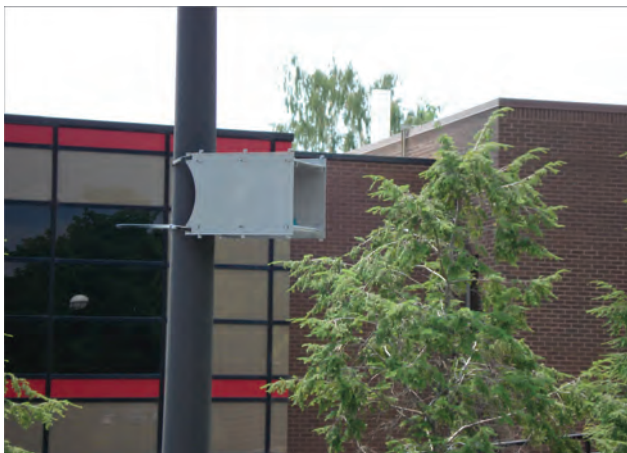
Outdoor shelter for suspending Radiello samplers for environmental/ambient air sampling.
