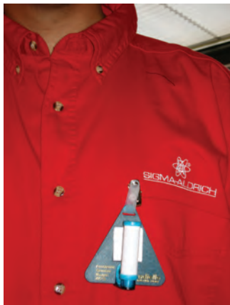
Personal monitoring (breathing zone assessment) of employees to hazardous substances.
