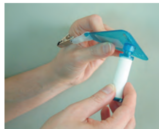
2a. Screw diffusive body into triangular support plate.
