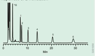
Analyzed with a Discovery C18 HPLC column, 15cm x 4.6mm ID, 5µm particles
