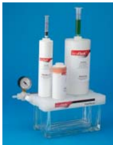
Figure 5. Loading Multiple VersaPak Cartridges
