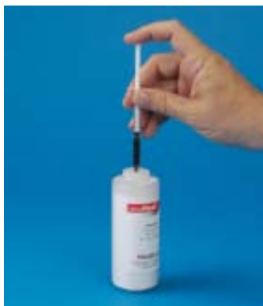
Figure 4. Direct Sample Loading Onto Cartridge
