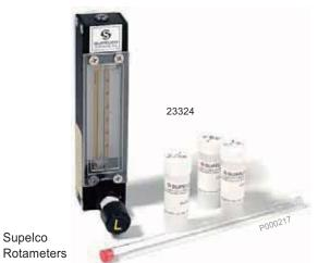
Designed for accurate metering, these rotameters are excellent chromatographic purposes. Each rotameter consists of a flow tu and four interchangeable floats. Standard flow tables (mL/min at STP) are included. The rotameter is easy to mount on any chromatograph, or you can install it on the optional tripod assembly. Available with or without needle valves.
