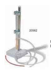
Use these bubble flowmeters to check splitter or detector flow, or to calibrate personal pumps for accurate air sampling. Bubble meters are graduated in these increments: 10mL by 1mL; 25mL by 5mL; 50mL by 10mL; 100mL by 20mL; 500mL by 50mL; and the 1000mL by 100mL. The 500mL and 1000mL meters can be used to measure positive or negative flow.
